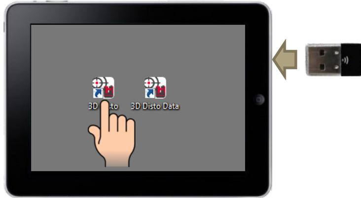
If a USB WLAN dongle is required, plug it in and start the 3D Disto software for Windows.
